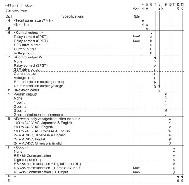
Note 1: Not available for the 7th code "C", "E", "P", "R", "S". However, if you want to order the 6th code "A" (SPST relay contact for the control output 1) and the 7th code "R" or "S" (current/voltage re-transmission output for the control output 2), specify the model as follows:
