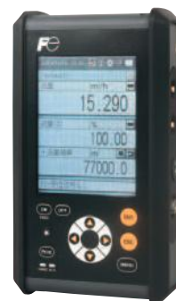
Flow transmitter (FSC)
