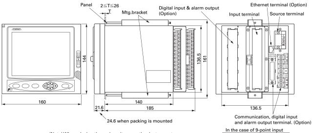
(Note) When placing the main unit on another instrument or on the floor, allow a space of 100mm or more between the unit and instrument or the floor.
